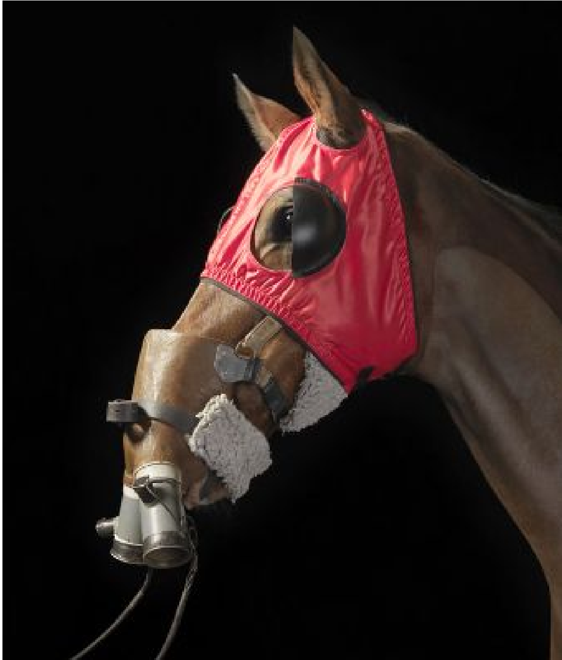
Mask - Respiratory Measurement Digital C-type.
